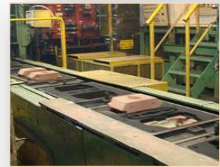
Horizontal moulding 800X600mm 2x250mm Green sand
